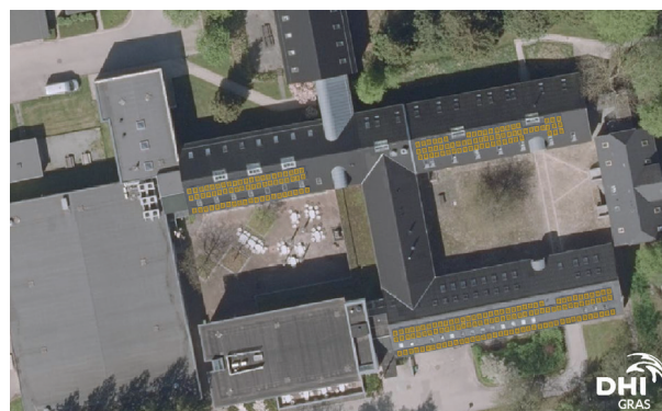
Deep learning approach to automatically segment solar cells on rooftops from very high-resolution satellite imagery.
